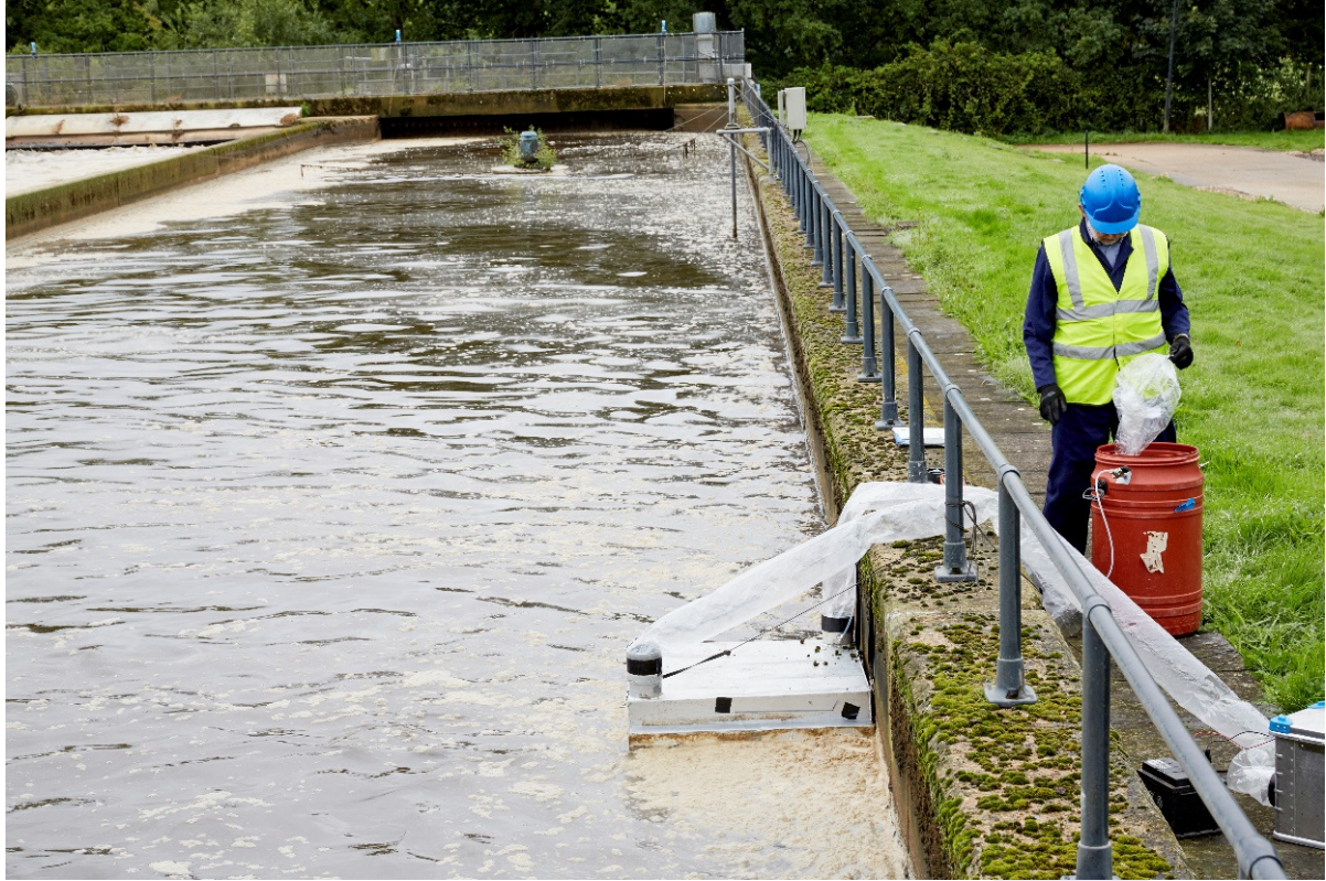
Figure 1 Sampling on the aeration lane with the Lindvall type sampling hood as used on tank surfaces in this study.
